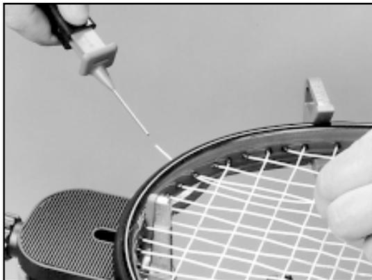
While holding pressure on the string, slowly pull the sheath out of the grommet hole to leave the end of the string exposed.
