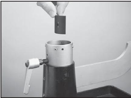
Place the brake pad into the turntable tube, then insert the end of the brake lever bolt into the hole of the brake pad so that the brake pad rests on the shoulder of the bolt.
