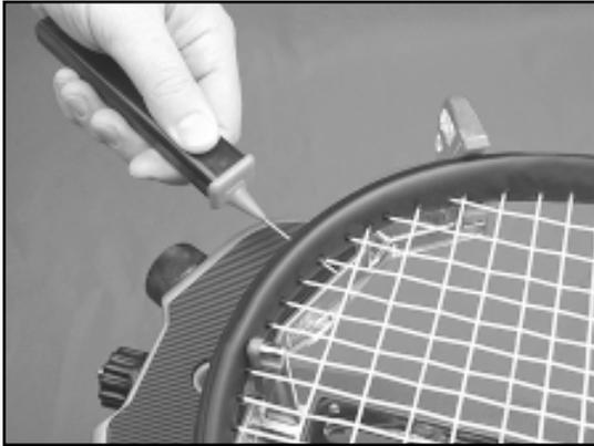
The Gamma 602 includes the new Pathfinder stringing awl which creates a pathway between or around strings to make inserting a string through tight grommets easier and quicker.
