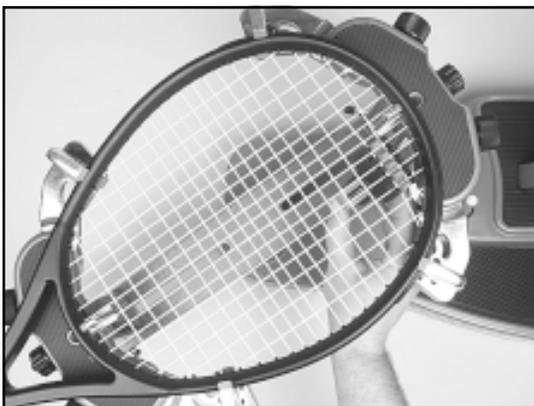
Weave the cross strings over and under the main strings being careful to alternate the weave of each consecutive cross string so as to be opposite of the previously installed cross string.
