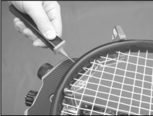
The Progression 600FC includes the new Pathfinder stringing awl which creates a pathway between and around strings to make inserting a string through tight grommets easier and quicker.
