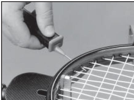
The Gamma 7000Es includes the new Pathfinder stringing awl which creates a pathway between or around strings to make inserting a string through tight gromets easier and quicker.
