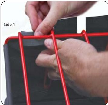
Step 10: On the side, separate the first hook and loop strip, and fold it over the first wire of the red Frame Assembly.
