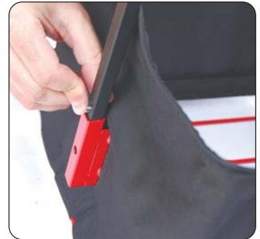
Step 12: On Sides 1 & 2, insert the handle into the red handle receivers, press the buttons in, and continue to push down until the silver button pops through the hole, securing the handle in place.
