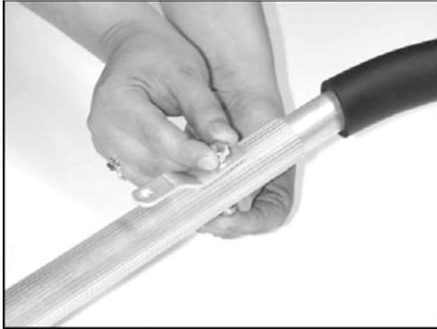
Step 1: Insert the ends of the Curved Handle into the open ends of the two Fluted Handles. Align the holes for the Hang Hooks, insert the longer two bolts then fasten nuts by hand on the bolts.
