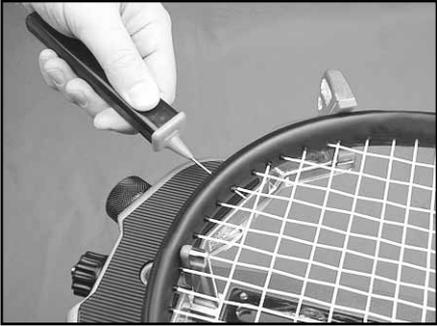
The machine includes the pathfinder stringing awl which creates a pathway between or around strings to make inserting a string through blocked grommets easier and quicker.
