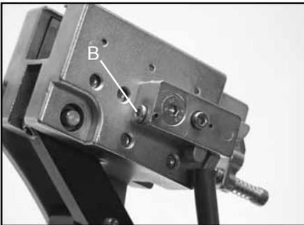
If the lever releases before 60 lbs., using the supplied L-shaped hex wrench, turn the adjustment screw (B) located on the left side of the latch block counter-clockwise to increase the engagement of the brake release latch with the brake lever. Repeat step 1 and adjust until the correct tension is indicated on the calibrator.
