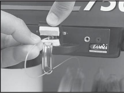
To measure out a length of string from a reel (sets can also be measured) insert one end of the string through the string guide grommet (from the backside). While lifting the clamp pad, insert the string through the entrance hole of the face plate until it appears at the exit hole and release the clamp pad. (The clamp pads will prevent debris from entering the SLM.)
