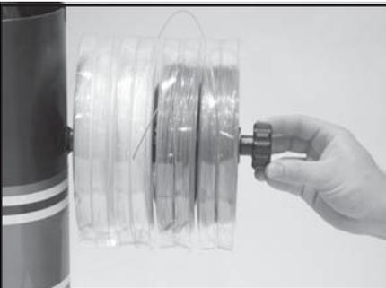
After the last reel is installed, place the remaining spacer(s) on the pin and attach the threaded knob to the end of the pin.
