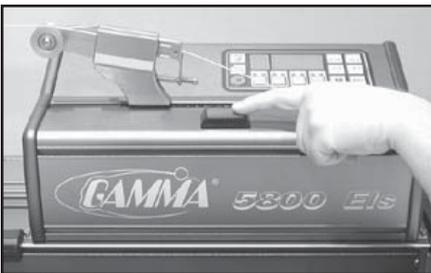
To tension a string, push the tension button or the foot pedal. The string gripper will move away from the racquet and slowly apply tension to the string. When the set tension has been attained, the gripper will stop moving. As the tensioned string stretches, the gripper may move intermittently, maintaining the set tension.
