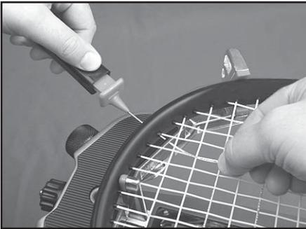
Once the awl is inserted, pull the handle of the awl outward while holding the tip section in place, leaving the outer sheath in the grommet hole.
