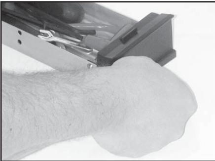
To open the drawers, reach under the right side end caps to find the the spring loaded latch handle. Pull the latch handle toward the outside of the end cap to release latch from
