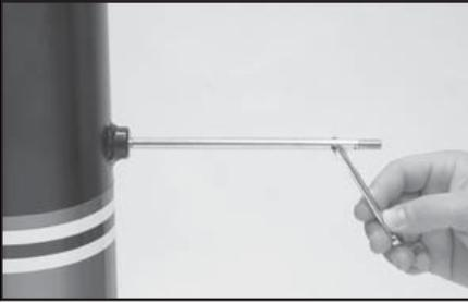
The string reel holder pin is an 8 mm rod with threads on both ends, and flat surfaces machined on one end. Thread the end of the pin without the flat surfaces into the threaded boss on the right side of the lower column support. Using the M6 open end wrench positioned on the flat surfaces, securely tighten the pin to the lower column support.
