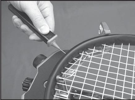
The machine includes the Pathfinder stringing awl which creates a pathway between or around strings to make inserting a string through tight grommets easier and quicker.
