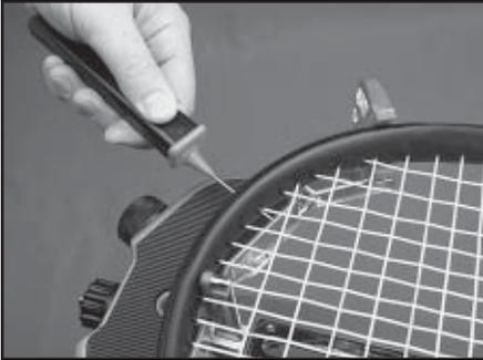
The GAMMA 6004 includes the Pathfinder stringing awl which creates a pathway between or around strings and through tight grommets.
