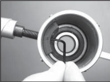
Insert the 2.5 mm L-shaped wrench into the flat head screw located on the inner side of the brake pad and the end of the brake lever bolt. While holding the locking lever bolt, turn the head of the screw counterclockwise with the wrench to loosen the brake pad. Carefully remove the turntable pad screw.
