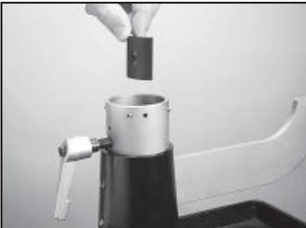
Place the new brake pad into the turntable tube. Insert the end of the brake lever bolt into the hole in the of the brake pad until the brake pad rests on the shoulder of the bolt.
