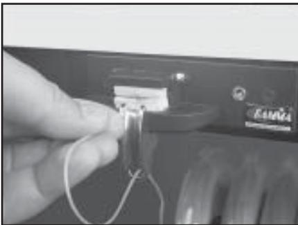
When the end of the string appears out of the exit hole, press the “C” button on the keypad to “Zero” the SLM, and the length of string measured will be measured from the point on the string located at the edge of the exit hole. Pull the end of the string in a slow steady fashion and the SLM will begin measuring the length of string pulled and indicate the measurement on the LED display. When the desired length of string is measured, cut the string at the exit hole.
