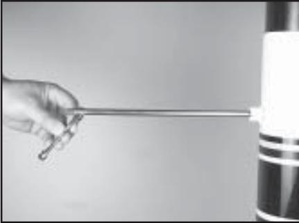
The string reel holder pin is an 8 mm rod with threads on both ends, and flat surfaces machined on one end. Thread the end of the pin without the flat surfaces into the threaded boss on the right side of the lower column support. Using the M6 open end wrench positioned on the flat surfaces, securely tighten the pin to the lower column support.
