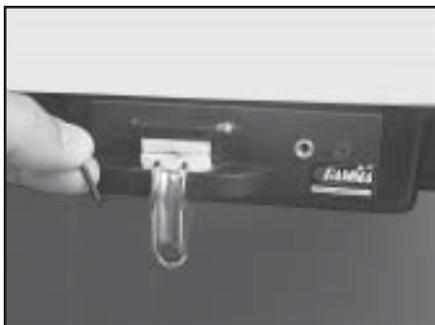
Position the face plate assembly over the opening in the bottom cover, and align the two countersunk end holes of the face plate with the threaded attachment holes in the front of the string length meter. With the two flat head machine screws, secure the face plate assembly to the string length meter.
