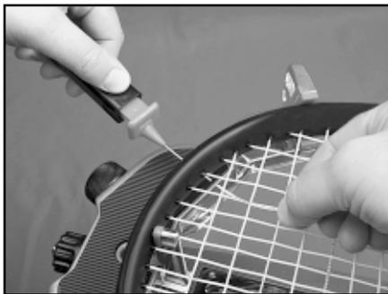
Once the awl is inserted, pull the handle of the awl outward while holding the tip section in place, leaving the outer sheath in the grommet hole. Insert the end of the string into the center of the sheath.
