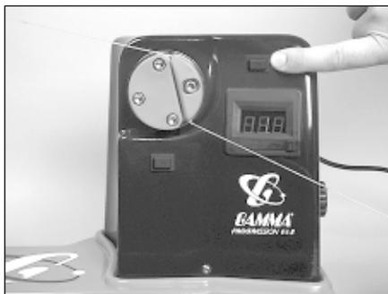
To tension a string, push the tension switch or the foot pedal. The string gripper will rotate and slowly apply tension to the string. When the set tension has been attained, the gripper will stop rotating. As the tensioned string stretches, the gripper may rotate intermittently, maintaining the set tension.
