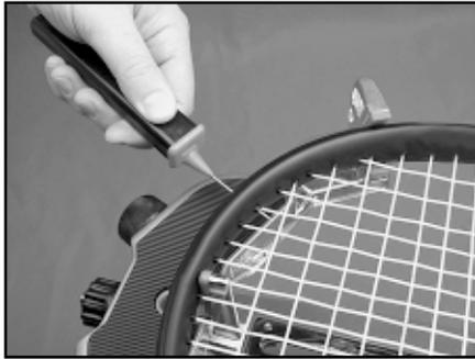
The Progression ESII+ includes the Pathfinder stringing awl which creates a pathway between or around strings to make inserting a string through tight grommets easier and quicker.
