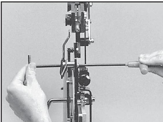
To tighten the braking mechanism, turn the set screw (A) counter clockwise by about 1/8 turn. Re-tighten the allen screw (B) on the back side of the tensioner frame and check for brake tightness. The tensioner should move freely along the track with the brake lever engaged and should hold tension with the brake lever released. If more adjustment is needed, repeat steps above until properly adjusted.
