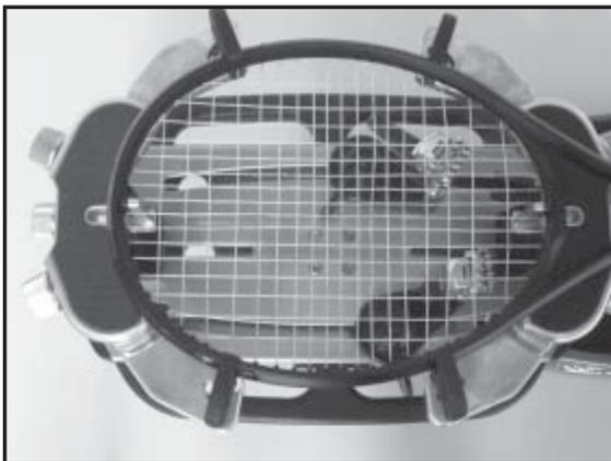
Once the final cross string is tensioned and clamped, tie off at the appropriate hole specified by the racquet manufacturer.
