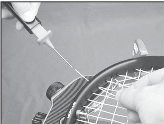
While holding the string, slowly pull the sheath out of the grommet hole to leave the free end of the string exposed.
