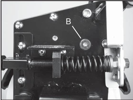
While holding the 6mm brake lever adjustment bolt (A), loosen the hex bolt (B) located on the back side of the tensioner frame with the 4 mm allen wrench.
