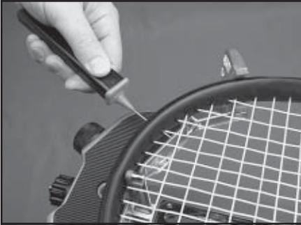
The machine includes the Pathfinder stringing awl which creates a pathway between and around strings to make inserting a string through tight grommets easier and quicker.
