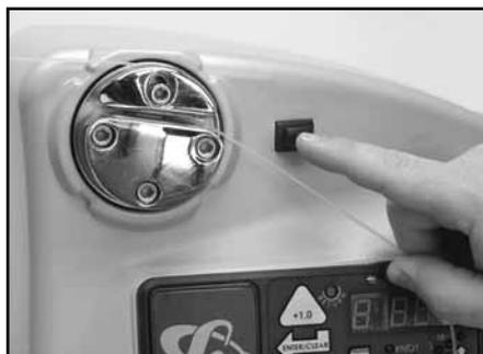
To tension a string, push the tension switch or the foot pedal. The string gripper will rotate and slowly apply tension to the string. When the set tension has been attained, the gripper will stop rotating and the display will flash. As the tensioned string stretches, the gripper may rotate intermittently, maintaining the set tension.
