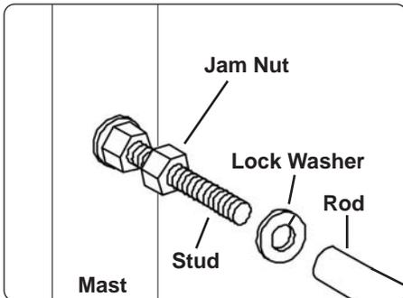
Step 1: Starting at the top, screw 1 Jam Nut onto the Stud until it is tight against the pre-installed Jam Nut. Place a Lock Washer on the Stud against the Jam Nut. Install 1 Score Card Rod onto the Stud until fully seated against the Jam Nut you installed. Align the Rod so loop openings are at the rear (see image on next page).
