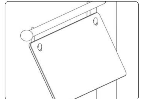
Step 3: Align the holes in the Name Card with the hook of the Name Card Rod. Apply gentle pressure to the card until it snaps into place on the hooks. The card may need to be tilted for installation.
