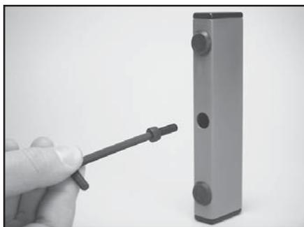
Place one screw onto the end of the 4mm hex wrench. Carefully insert the screw through the large hole in the bottom of the leg and continue through the small hole at the top of the leg.
