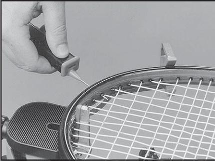
The GAMMA 600ES includes the new Pathfinder stringing awl which creates a pathway between or around strings to make inserting a string through tight gromets easier and quicker.
