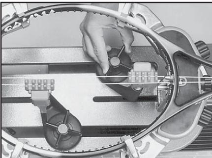
Secure the tensioned main string using the remaining fixed clamp. Repeat the procedure for all of the remaining main strings and tie off following the racquet manufacturers recommendations.
