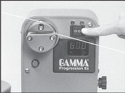
Push the Tension Switch toward the right side of the machine. The string gripper will rotate and slowly apply tension to the string. When the set tension has been attained, the gripper will stop rotating and the green LED will light. As the tensioned string stretches, the gripper may rotate intermittently, maintaining the set tension.
