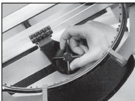
Rotate the winged lock knob clockwise to secure the clamp base to the turntable.
