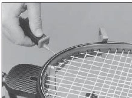
The Gamma 600 includes the new Pathfinder stringing awl which creates a pathway between or around strings to make inserting a string through tight gromets easier and quicker.
