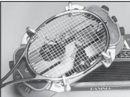
Weave the cross strings over and under the main strings being careful to alternate the weave of each consecutive cross string so as to be opposite of the previously installed cross string.
