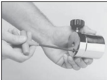
The drop weight is of a two piece design. When assembled, it will accommodate tensions from 20 lbs. to 90 lbs. For tensions from 8 to 20 lbs., remove the 5mm bolt on the face of the drop weight, and use the smaller portion of the weight as described above.
