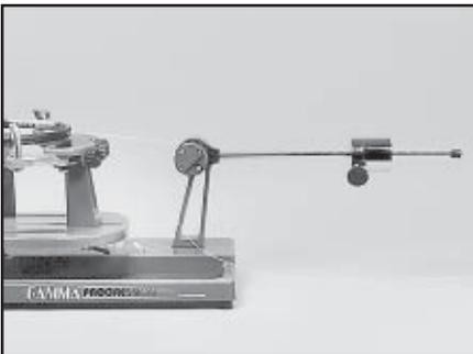
When the correct tension is attained, the drop weight bar will rest horizontally as shown. For accurate tensioning, it must be lowered and come to rest at horizontal without assistance. Manually forcing the tension bar to the horizontal position will greatly increase the string tension and may result in racquet damage.
