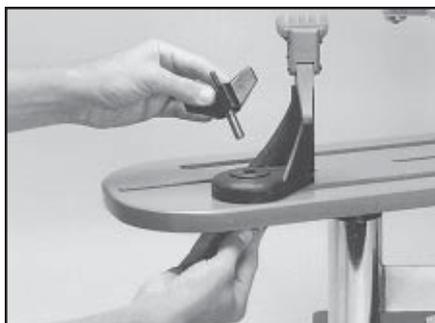
Place the load bushing into the top of the clamp base mating it to the lower guide bushing. After checking that the thrust bearing is positioned correctly in the base of the winged lock knob, screw the knob into the base bushing until fully seated.
