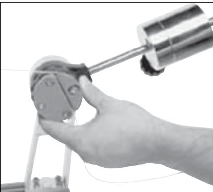
While holding the string gripper drum with your hand, lift the tension bar to approx. 45 degree angle and let fall. If the tension bar drops below horizontal, repeat the above action until the bar comes to rest parallel to the racquet. The set tension will be reached when the bar rests horizontal.
