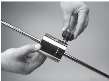
To set the stringing tension, loosen the locking knob on the side of the drop weight. Slide the weight in the appropriate direction until the face **closest** to the string gripper is indexed with the desired tension mark on the tension bar.
