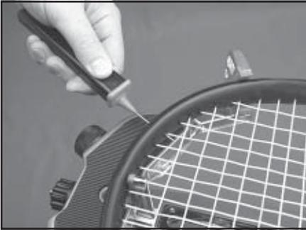
The Gamma X-6 includes the Pathfinder stringing awl which creates a pathway between or around strings to make inserting a string through tight gromets easier and quicker.
