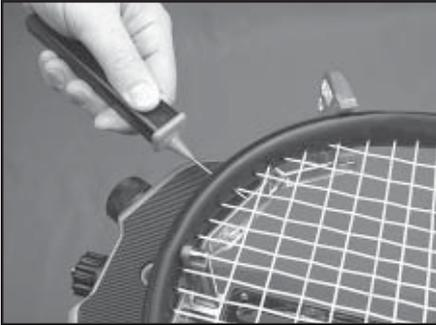
The stringing machine includes the Pathfinder stringing awl which creates a pathway between or around strings to make inserting a string through tight grommets easier and quicker.
