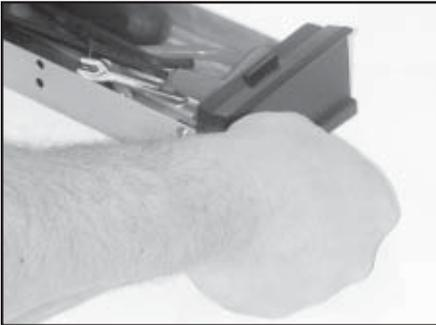
To open the drawers, reach under the right side end caps to find the the spring loaded latch handle. Pull the latch handle toward the outside of the end cap to release latch from the end cap and slide the drawer out.
