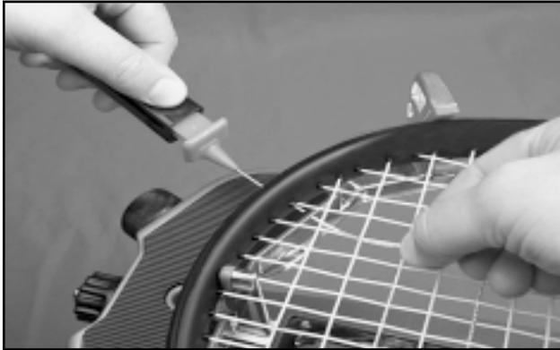
Once the awl is inserted, pull the handle of the awl outward while holding the tip section in place, leaving the outer sheath in the grommet hole. Insert the end of the string into the center of the sheath.
