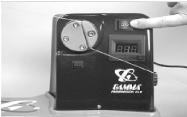
Push the Tension Switch toward the right side of the machine. The string gripper will rotate and slowly apply tension to the string. When the set tension has been attained, the gripper will stop rotating. As the tensioned string stretches, the gripper may rotate intermittently, maintaining the set tension.
