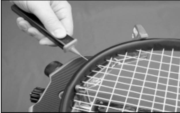
The Progression ESII includes the new Pathfinder stringing awl which creates a pathway between or around strings to make inserting a string through tight grommets easier and quicker.
